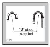
Place the drain hose into your standpipe, which should have an internal diameter of approximately 38mm thus ensuring there is an air break between the drain hose and standpipe.
